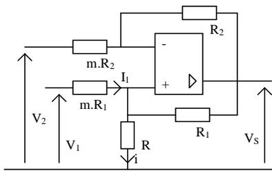
$$V_- = \frac{V_2/mR_2 + V_S/R_2}{1/mR_2 + 1/R_2} = \frac{V_2 + mV_S}{1 + m}$$
