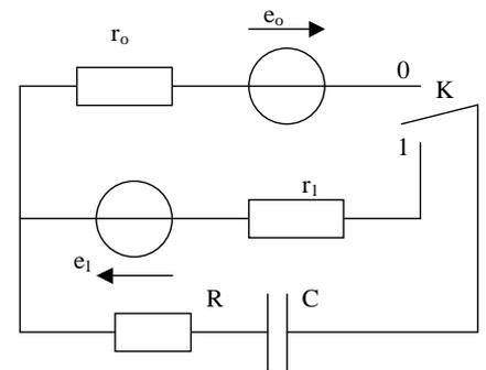
$$R : t_1 = \tau_0 \ln 2. \quad q(t) = C e_0 (1 - \exp(-t/\tau_0)) ; \quad q(t) = (C e_1 + C e_0 / 2) \exp(-(t-t_1)/\tau_1) - C e_1. \quad i = dq/dt.$$
